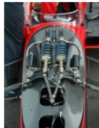
Figure 9. An inboard suspension system on a CART car. (World Wide Web)
