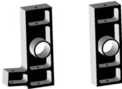
Figure 34. Suspension uprights. Left image is rear upright. Right image is front upright.
