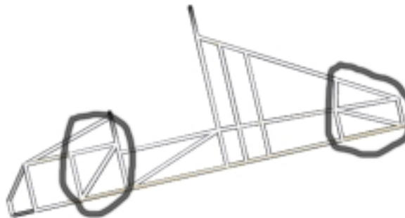
Figure 3. Side view of the frame identifying suspension mounting locations.
